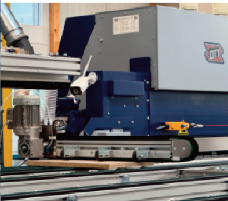
► At Paul Ott, the furniture panels are cleaned on the edge-processing line using a Wandres Microfilament Sword Brush.
