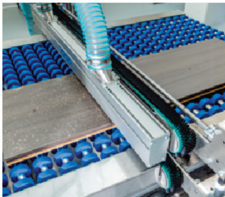
► A Trans-Vac Unit TKL 46 can be installed upstream for pre-cleaning to remove coarse debris before it reaches the brush.
