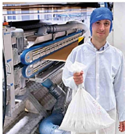
Stephan Leu, technical director at Wandres, evaluated the extracted dust quantity at regular intervals. The test setup was able to remove enormous amounts of paper dust from the web.
