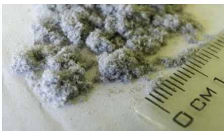
Fig. 1: Large quantities of dust are created during transport and cutting processes
