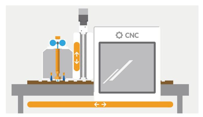
▶ The cleaning machine and the CNC machine are connected by a vertical adjustment unit. The horizontal axis of the CNC machine is used during the cleaning process. (Image is not drawn to scale)
