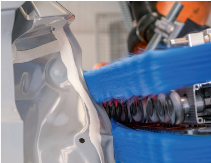
The brush filaments follow the geometry of the vehicle precisely without ever touching the wet seam sealing.
