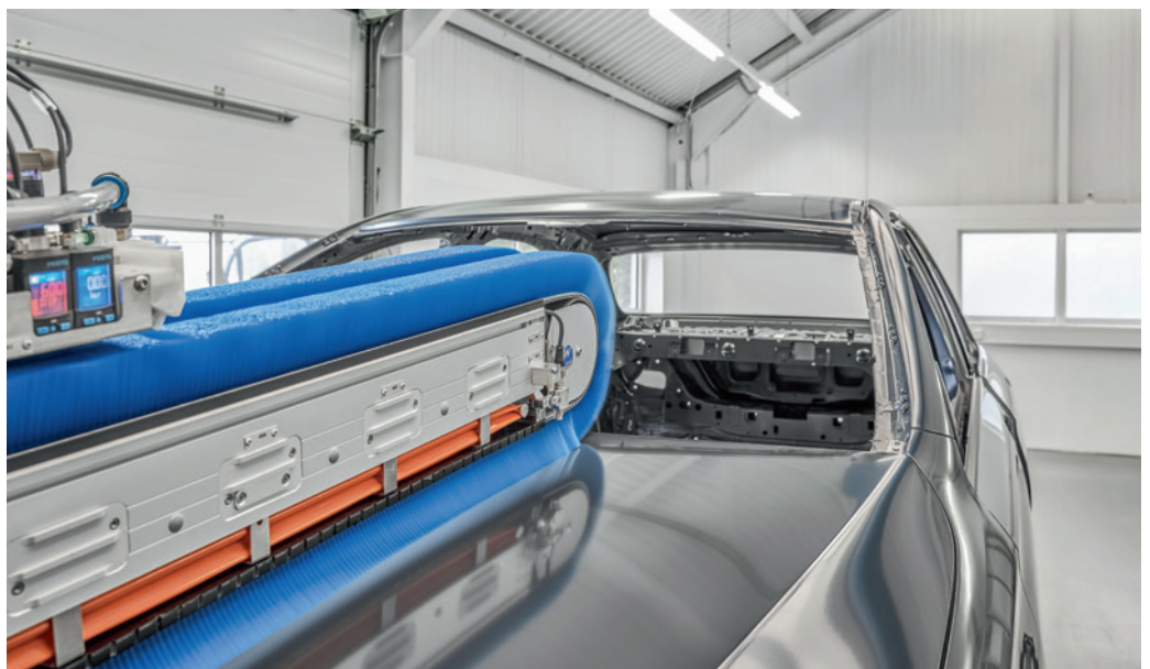
A bodyshell is cleaned and the procedure tested in the Wandres Technology Centre.
