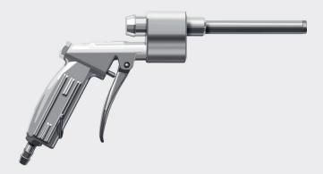
**The Suction Gun..** is ideal to effectively remove non-toxic particles and short chips. The suction air flow functions according to the Venturi principle: Compressed air passes a ring nozzle thus creating a vacuum within the suction tube. The incoming air conducts the particles and chips towards the exhaust air hose. Suction performance may be regulated infinitely via a hand lever.
