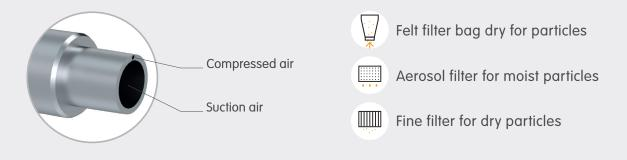
The **Vac-Blast Cleaner** is ideal to remove non-toxic particles and short chips. The suction air flow functions according to the Venturi principle: Compressed air passes a ring nozzle thus creating a vacuum within the suction tube. The incoming air transports the particles and chips towards the exhaust air hose and the debris container.
