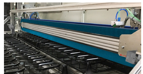
Cleaning of injection-moulded parts on a tray
