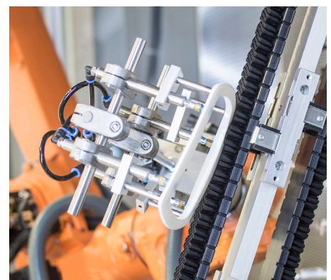
Robot-guided cleaning using a Sword Brush installed in fixed position
