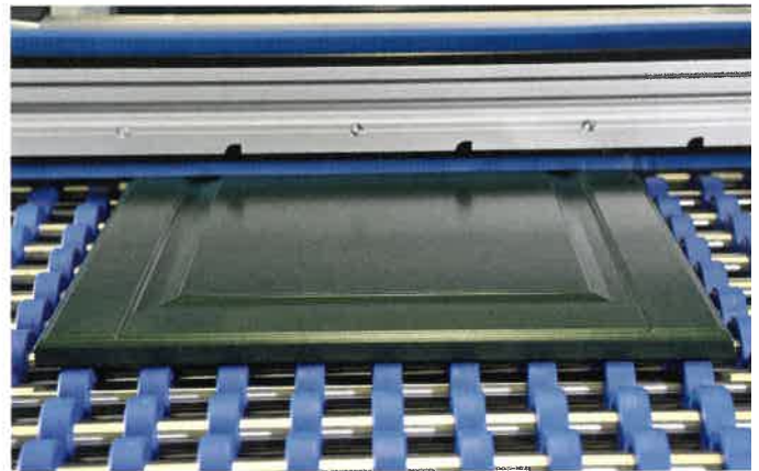
To achieve the best possible cleaning result, a Sword Brush removes residual fine dust following cleaning with air technology
