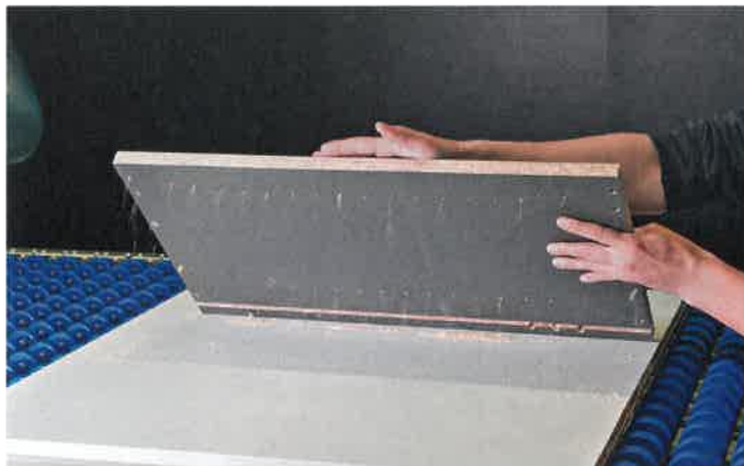
A knocking test dislodges substantial amounts of particles from bore holes prior to cleaning
