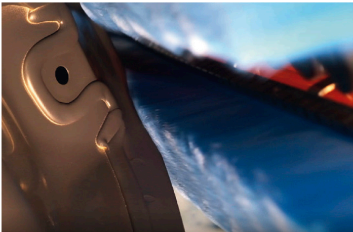
Freshly applied PVC seam sealing remains untouched by the brushes and is cleaned instead by Tornado Nozzles using air technology.
