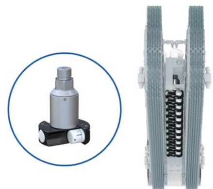
Tornado Nozzles Type Janus 50 D are mounted between two linear brushes
