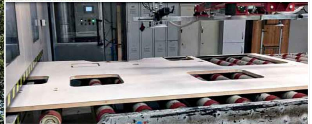
The sandwich panel was cleaned perfectly within a few seconds. Small details on edges and in grooves have now become visible.
