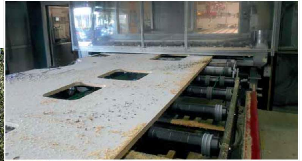
A wall panel with cut-outs for windows before cleaning (Image: Wandres)
