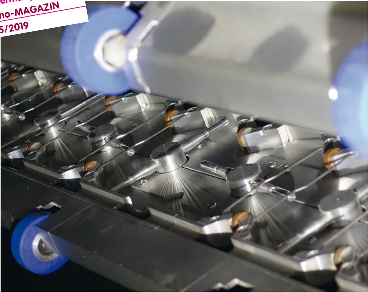
Air-assisted cleaning unit, view of rotating nozzles in the Tornado Channel
