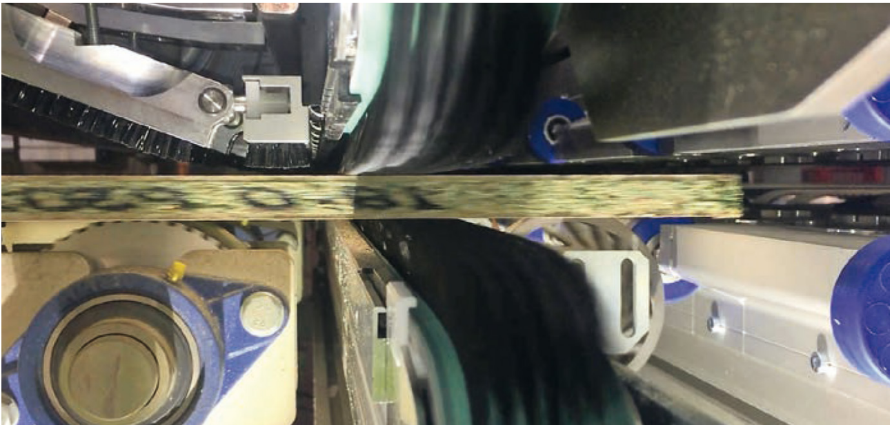
Cleaning chipboard from above and from below: touch control elements are visible on the left of the image, adjacent two Sword Brushes and to the right the upper and lower Tornado Channels
