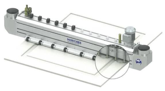
short brushes which are installed vertically and wipe the panel edging clean from top to bottom. A manual or electrical adjustment unit provides for adjustment to the panel width. This cleaning solution also allows for subsequent integration of the module into a roller conveyor line, ideally before panel surfaces are cleaned.
