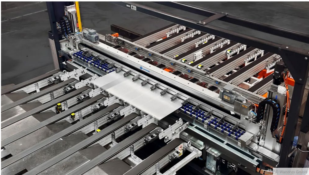
The Evomat EVO 501 cleans blanks in front of the press at high transport speed.
