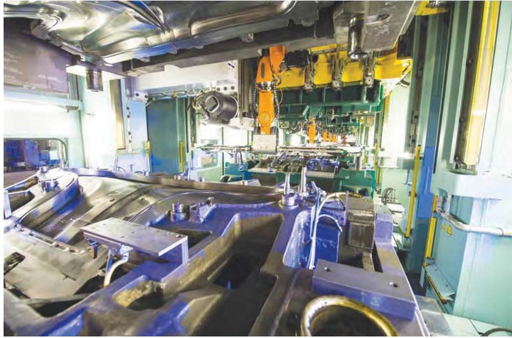
XL servo press in the Mercedes-Benz plant in Kuppenheim (Image: Mercedes-Benz)
